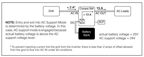
Figure 1-6 Regular AC Support without Xanbus Devices
