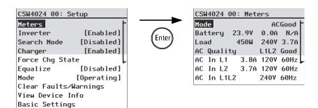
Figure 3-6 Viewing the Meters Screen
