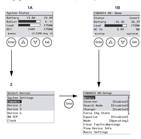
Figure 3-7 Navigate To Conext SW Setup Menu
