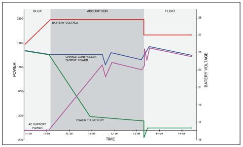
Figure 1-5 Enhanced AC Support Charge Cycle
