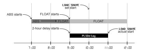
Figure 1-7 Load Shaving 2-Hour Delay Example
