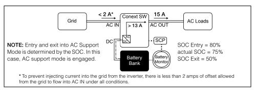
Figure 1-3 AC Support Mode using SOC
