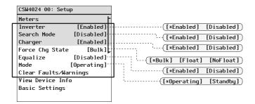
Figure 3-8 Conext SW Setup Menu Operational Settings
