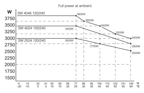
Figure 6-1 Output Power versus Temperature Derating Graph
