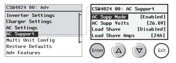
2. Set the battery voltage threshold for AC support mode to engage.
