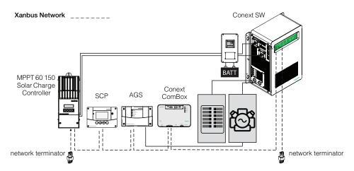
Figure 2-1 Xanbus System Components
