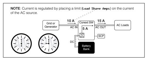
Figure 1-2 Load Shaving in Action
